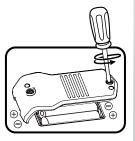
5. Replace the battery cover and tighten the screw to secure.
